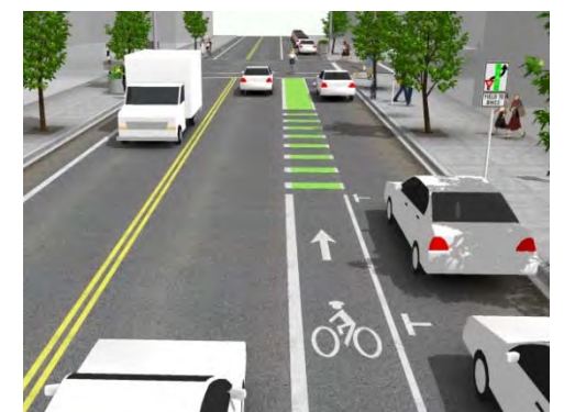
Green Bike Lanes through Conflict Areas
